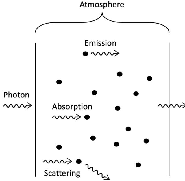
**Figure 2:** Schematic representation of three processes of radiative transfer.
